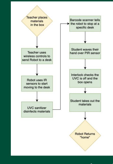
Figure 3: Example Flowchart of Robot's Functionality
